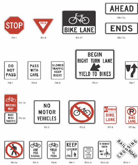
Figure 5. Regulatory signs for bicycle facilities
